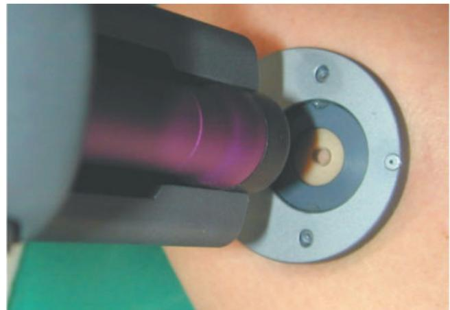
Fig. 5. Cooling device used with the Athos Nd:YAG laser. This device is composed of a sapphire plate drilled by a hole of 2 mm of diameter and surrounded by a steel duct chilled by a cryogenic gas. The cooling temperature was set at  $+5^{\circ}\text{C}$ .
